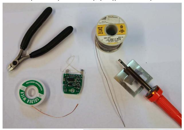
Using the de-soldering wick, I removed the solder from the two pads using short application times and allowing the tabs to cool a bit before removing more solder. Part to reason for the extra care here, in addition to concern about overheating the adjacent electronics, is that these tabs are tied to a lithium battery. It is **never** a good idea to overheat a lithium battery!
